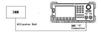
3. Select Sine waveform of the generator and set the amplitude to the values listed below in sequence.
