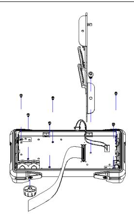
6. Remove the keypad circuit board assembly.
