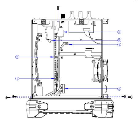
4. Separate the front panel from the main body of the generator.
