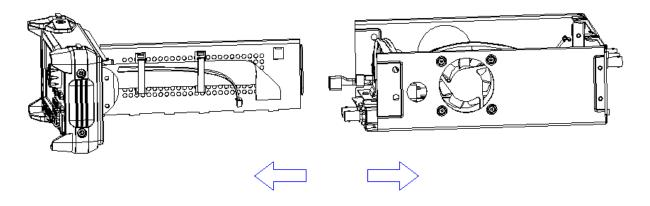
5. Pull out the knob and then remove the screws attaching the hardware partition plate and the front cabinet screws.
