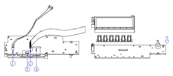
9. Remove all the 9 screws fixed the main board and power supply board using the T10 Torx screwdriver and separate the main board and power supply board carefully from the main body of the generator to avoid being scratched by the sharp metal edge.
