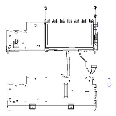
8. Pull out the connecting cable according to the index number as shown in the following figure and remove the keyboard.
