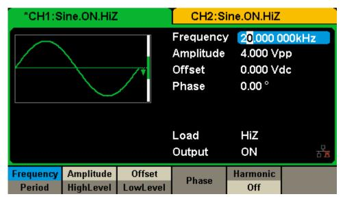
**Note:** The desired numerical value can be modified using the knob and direction keys.
