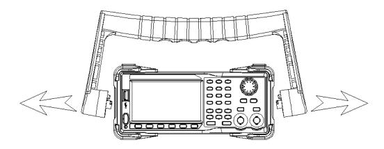
After removing 4PCS screws of the pad and 1PCS screw at the bottom of the generator's case, remove the metal shell carefully from the main body to avoid being scratched.
