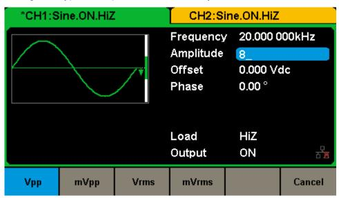
Then press the corresponding softkey to select the desired unit. For example, press **Vpp**.
