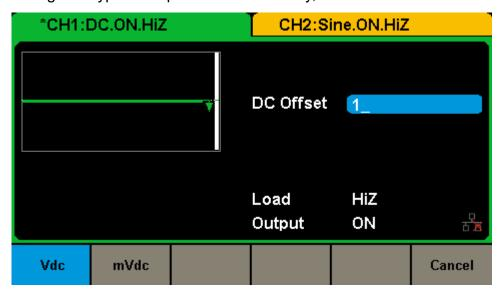
Then press the corresponding softkey to select the desired unit. For example, press **Vdc.**
