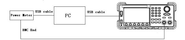
3. Select Sine waveform of the generator and set the amplitude to 1 V and 2.5 V, frequency to the values listed below in sequence.
